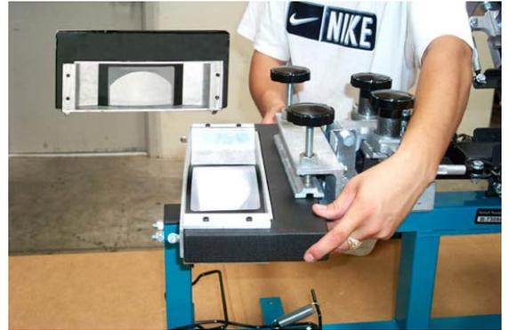
If necessary, use spray adhesive on the cap platen to help hold the cap in position. Place the cap over the cap platen and lift the spring loaded cap hold down.
