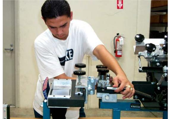
After the screen has been micro adjusted, securely tighten the micro adjustment knobs before printing.
