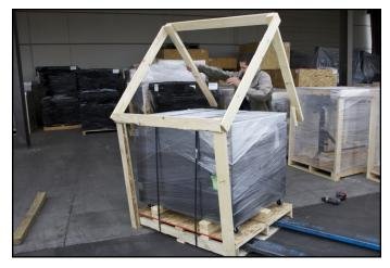
3. With two people lift the SD-10 and place it into the desired location. Cut the banding and remove all of the plastic wrap. Plug the unit into a grounded wall outlet.
