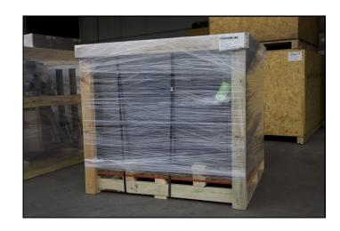
2. Remove the side rails first followed by the rest of the outer frame.
