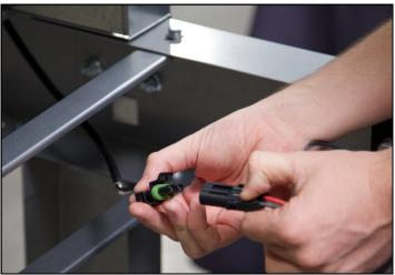
4. Connect the plug located inside of the machine to the plug connected to the motor located on the arm.
