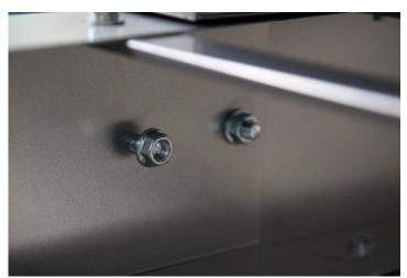
3. Thread a lock nut onto the other side of the bolt, which is located inside of the dryer. Repeat steps 2-3 to install the other three holes.
