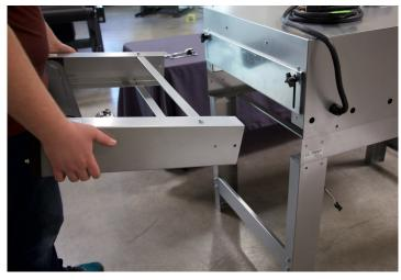
1. The side without the wire is the side that the infeed is installed into. Slide the arms (without the motor) into the base, while aligning the holes of the arm and the base.
