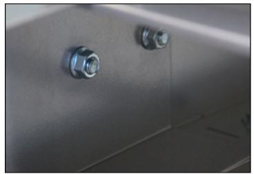
3. Thread a lock nut onto the other side of the bolt, which is located inside of the dryer. Repeat steps 2-3 to install the other three holes. Do not tighten the nuts and bolts with wrenches until the belt is installed.
