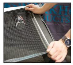
3. Thread the belt until both ends meet on the outfeed roller.
