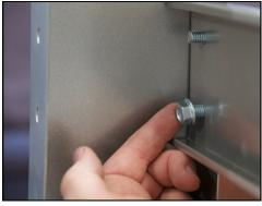
3. Insert a washer and a hex nut onto the other side of the bolt. Tighten it by hand. Repeat for the other seven bolts.
