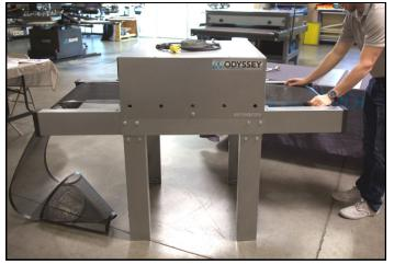
1. Thread the belt over the top of the infeed roller and over the upper cross brace. After the belt has gone through the chamber, pull the belt to hang over the outfeed roller to add weight to help with the threading of the lower portion.
