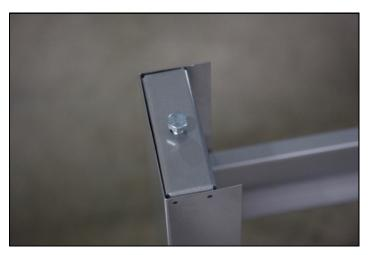
4. Turn the legs are and insert the leg levelers onto the four legs.
