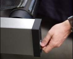
4. To install the belt it may be required to adjust the belt tracking. This is done by turning the tension bolt clockwise (to tighten) or counterclockwise (to loosen). Belt tracking will be explained more in-depth on page 11.
