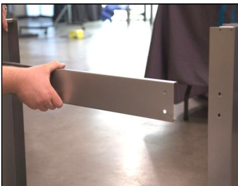
1. Align the holes of the cross base with the holes on the bottom of two legs. The backside of the cross brace should face out, and the inside of the brace should face in.
