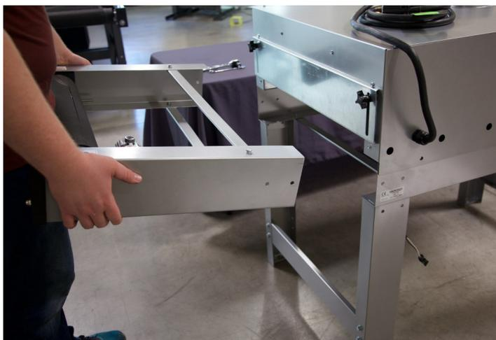
1. The side without the wire is the side that the infeed is installed into. Slide the arms (without the motor) into the base, while aligning the holes of the arm and the base.
