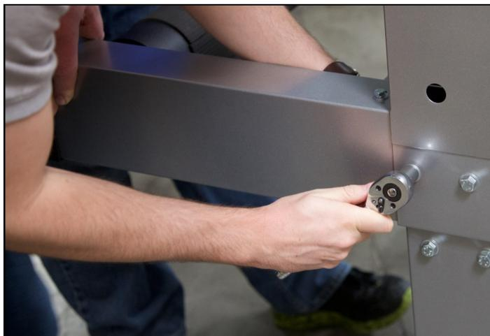
4. Using a wrench for the inside nut and a socket for the outside bolt, tighten the nut and bolt to hold in place. Tighten the other three bolts and nuts, leaving them loose enough to adjust for leveling.
