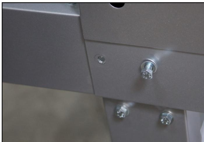
2. Insert a washer and hex bolt into one of the holes that connect the base and the arm.
