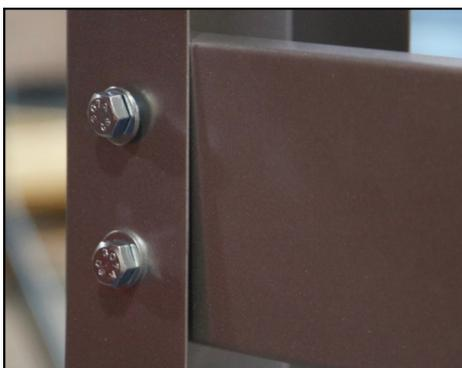
2. Insert a washer and a hex bolt (3/8-16" x 3/4") into the top holes. Hand tighten a lock nut onto the other side of the bolt.
