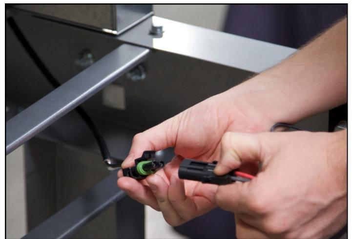
4. Connect the plug located inside of the machine to the plug connected to the motor located on the arm.
