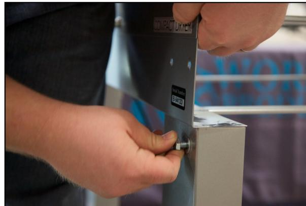
7. With the holes of the base and the leg aligned, insert a washer and hex bolt into the outer hole.
