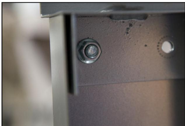
8. Tighten a lock nut onto the other side of the bolt, which faces inside the dryer. Only hand tighten it.
