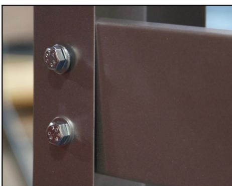
2. Insert a washer and a hex bolt (3/8-16" x 3/4") into the top holes. Hand tighten a lock nut onto the other side of the bolt.
