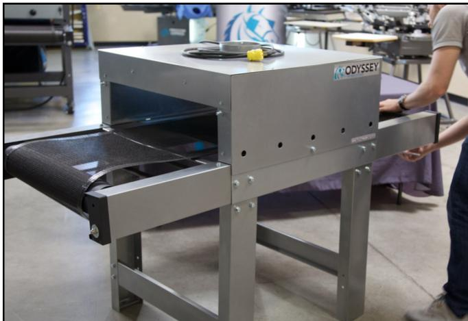
2. On the infeed side, take the other end of the belt and thread it under the infeed roller and under the lower cross brace, through the lower slot on the roller/rail assembly. Guide the belt through the oven chamber so it continues through the lower slot and over the lower cross brace.
