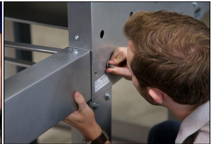
2. Insert a washer and leg bolt into one of the holes that connect the base and the arm.
