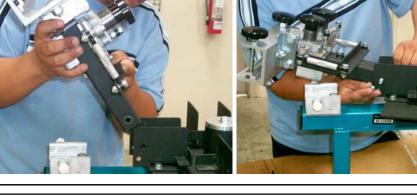
Tighten the top bolt using two 1/2" wrenches.
