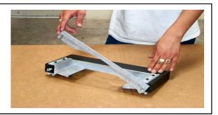
Bend the screen slightly until it fits the contour of the two slots on either side of the ink well.
