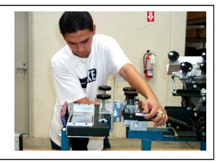
After the screen has been micro adjusted, securely tighten the micro adjustment knobs before printing.
