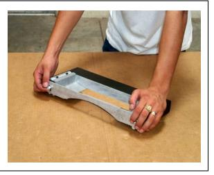
Lift the gate from the side that has the slot.
